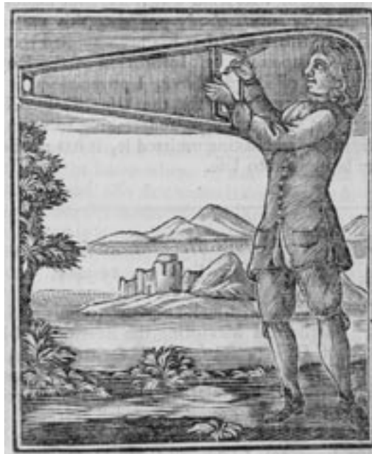
Figure 4: Hooke's portable camera obscura (1694).
