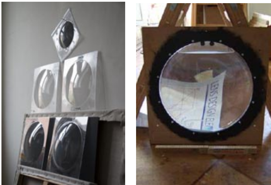
Figures 3a – b: Water Lenses II a: Self-manufactured spheres of plexi-glass which form the convex side of a water lens. b: Self-manufactured plano-convex water lens. Diameter: c. 380 mm, focal length: c. 1100 mm.
