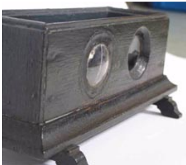
Figure 2b: Water Lenses I – Simple water lenses in the 17th century could have looked like these ones that consist of convex plate glasses made of hollow glass and flat sheets of glass, stuck with putty into wooden frames or boxes.
